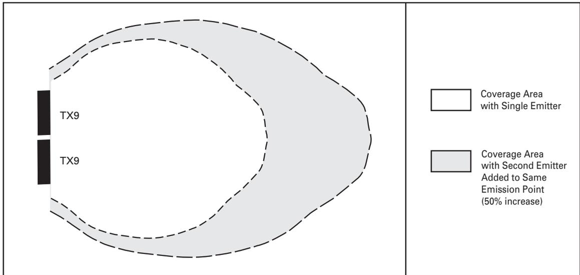
When two emitters are used at the same emission point in single channel mode, the overall coverage area increases 50%. When using an RX22-4 receiver, as a result, the coverage area will increase to an estimated 42,000 ft<sup>2</sup> (3,902 m<sup>2</sup>); the RX14-2 will increase to 5,250 ft<sup>2</sup> (488 m<sup>2</sup>); the RX16 will increase to 4,590 ft<sup>2</sup> (426 m<sup>2</sup>).
